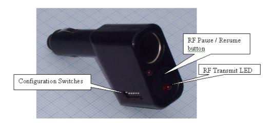
The VA is designed to plug into the Auxiliary Power (Cigarette Lighter socket) connecter available in virtually all cars and also has a spare socket for other plug-in items such as mobile phone chargers.
